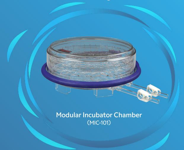
The Modular Incubator Chamber is a compact and versatile tool designed as a cost-effective system for maintaining cell cultures under stable hypoxic (physioxic) or hyperoxic conditions. It offers a straightforward approach to controlling oxygen levels using its closed system, preventing multi-well plate edge evaporation, and tailoring gas concentrations to your specific requirements.
